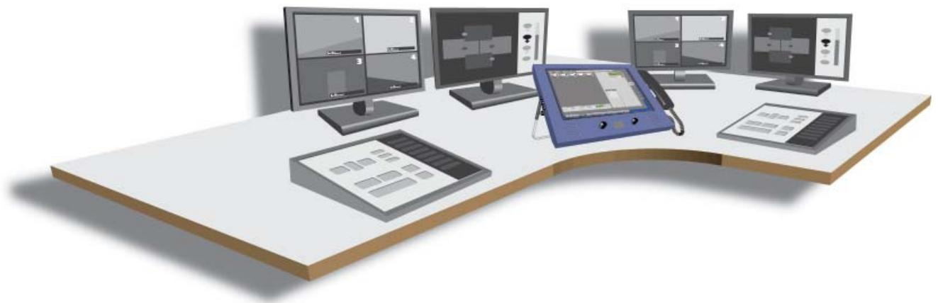
The command centre takes in calls from the sites and these are routed to the traffic manager. The traffic manager answers these calls and passes them to one of the operators. The operator will handle all voice and control actions necessary to regulate traffic. The CCTV cameras provide the operator with a good view of the situation on the road and waterway.
